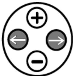
Press either left (←) or right (→) control button to **access each specific Function page**. You can press and hold either button to scroll quickly.
