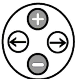
Press either the increment (+) or decrement (-) control button to see/change numeric value of any function. You can press and hold either button to edit numbers quickly.
