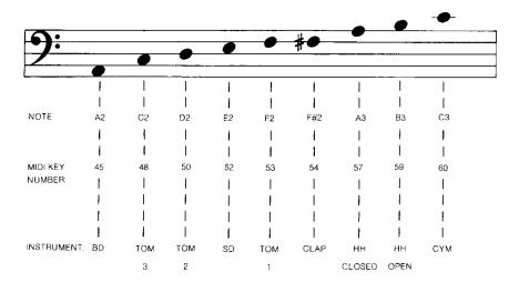
A key number transmitted by any MIDI synthesizer, sequencer or music computer will activate any RX21 instrument. For example, you can manually "play" the RX21 "drum kit" on a MIDI keyboard:
