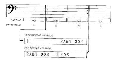
Having located the repeat sign, press DELETE, and the LCD will show "DELETE REPEAT?", then press  $\pm 1/YES$  to delete, or  $\pm 1/NO$  to cancel the delete function.
