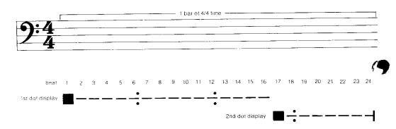
Just remember that the pairs of vertical dots indicate the primary beats in each bar, and you'll find that the Dot Display is a valuable aid for programming your RX21 rapidly and accurately in the step write mode. You can exit the step write mode from the Dot Display in the usual manner, by pressing the STOP/CONTINUE key.
