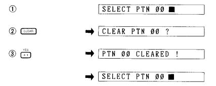
All programmable patterns in the RX21's memory (numbers 00-55) can be cleared simultaneously if required. This is a "hidden function" in the sense that it cannot be accessed directly—in order to prevent accidental erasure of the entire memory contents.
