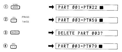
You can also delete repeats within a song, without losing any parts. See the DE-LETING REPEATS section for an explanation of this simple procedure.
