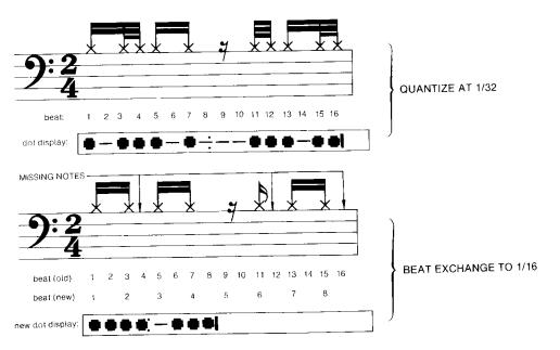
All the notes originally occurring on even-numbered beats have gone—permanently. It is safer, then, to use the Beat Exchange function for switching from a lower quantize rate to a higher one, so that you can add rhythmic subtleties rather than remove them.
