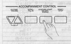
To begin with an introduction, press the INTRO button while in Synchro Start mode. As soon as a note or chord is played in the left-hand section of the keyboard the Intro will start.
