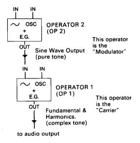
Operators do not have to be connected "vertically" in a modulator-carrier relationship, as shown above. The outputs of two operators can also be mixed—just as the stops in an organ are mixed. In this case the sounds are simply added together with no modulation effect.
