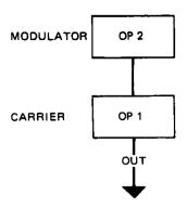
Most algorithms have multiple modulators and carriers. In one algorithm a given operator may be a carrier, while in the next it might function as a modulator—the only difference being how it is connected. In algorithm number 5, for example, there are two vertical stacks of two operators, and the outputs of the carriers in these stacks are connected in parallel (horizontally). Algorithm 5 has an equal number of modulators and carriers—two modulators and two carriers.
