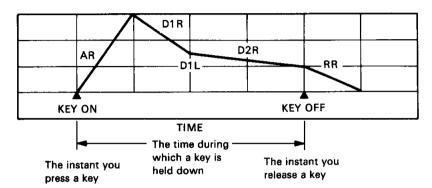
This envelope diagram can be used as a guide in visualizing the DX27/27S envelope settings while you program or edit a voice.
