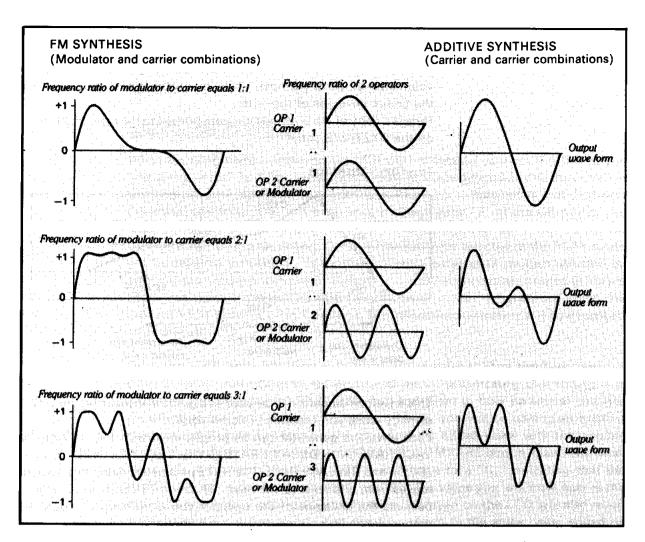
Still more variations can be achieved by changing the relative output levels between operators; the greater the level of the modulating operator, the more harmonics are present.
