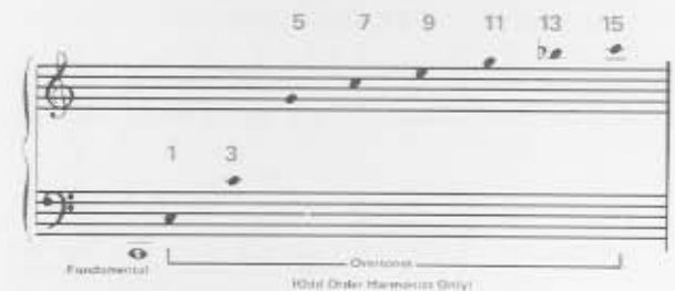
50% Square Wave Pulse Width
