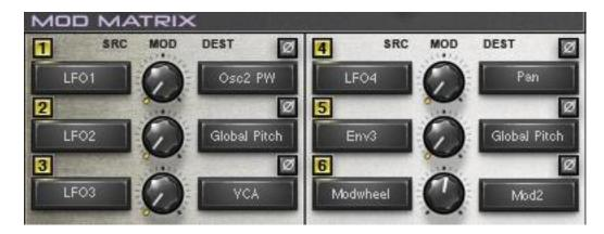
The Modulation Matrix allows the patching of modulation sources to selectable destinations.
