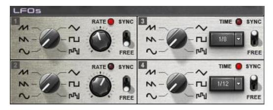
Element 2.0 features four identical LFOs that can be either free-running or synced to both MIDI clock and Note On commands.
