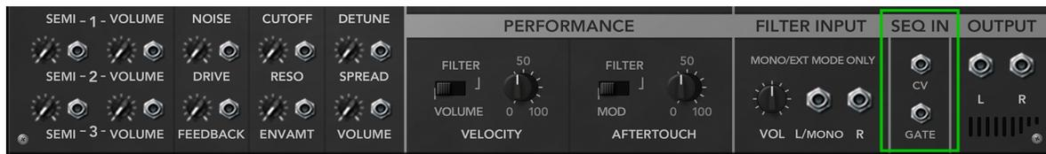
The sequencer inputs can be used to connect Reason's step sequencers (such as Matrix, RPG-8, or Thor's) to program monophonic note sequences using Gate/CV signals. For best results, the Polyphony mode switch on the front panel should be set to either "Mono/Ext" or "Unison". The Note Priority switch on the back panel should be set to "Last".
