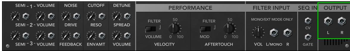
This section hosts the stereo output of The Legend. For monophonic applications, use the left (L) connector.
