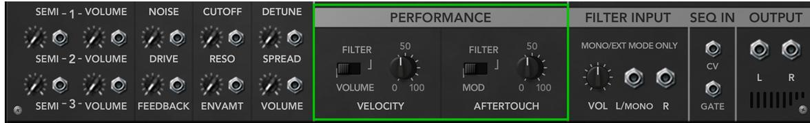
The Legend can respond to Velocity and Aftertouch by adjusting the controls in this section.
