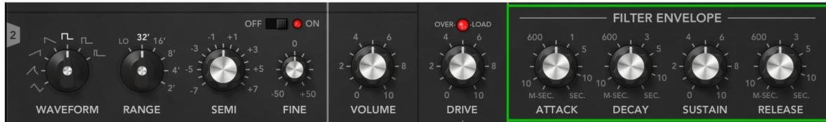
An envelope controls a sound parameter over time, starting from the instant a key is pressed (see fig. 3.2.8). The filter envelope is designed specifically to modify the filter cutoff frequency over time. Most sounds, whether synthetic or acoustic, start out very bright then become dark quickly. The filter envelope achieves precisely this effect in combination with the lowpass filter.
