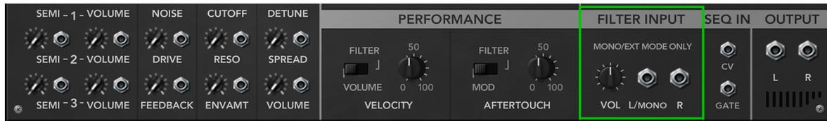
External sources (both mono and stereo) can be routed into The Legend using the Filter Input jacks, in order to take advantage of its high-quality low-pass filter. The level of the signal can be controlled with the Volume knob next to the input jacks.
