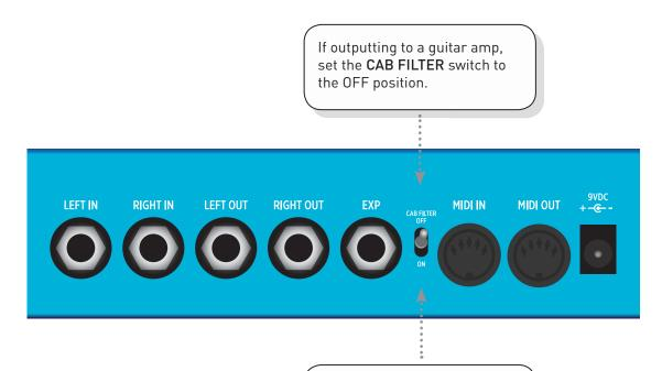
If outputting to a full-range PA system, recording interface, or headphones, place BigSky last in your effects chain and set the **CAB FILTER** switch to the ON position. This will engage our sophisticated speaker response curve. Your dirt pedals will sound amp-like, and your clean guitar will have a present yet rounded response even without an amp.
