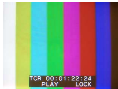
Timecode burn-in window in a video image.
