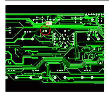
The square Pad is now the DC Signal input for PWM. It ranges from -3.8V to 2.3V for 0% to 100%PWM or you if want to use the range 50% to 100% (the 0% to 50% do sound exactly the same), -0.75V to 2.3V.
