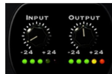
Figure 3: Output LED indicating maximum signal level
