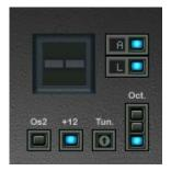
A speciality of old ob synths was that they had two vertically working levers instead of the popular wheels invented by moog. The **modulation lever** is on the left side. In the original it only worked downwise. In the OP-X, it can be used up- or downwise. Upwise, the modulation is inverted (hearable only in a realtive time context). The **pitch lever** is on the right side. It reacts vice versa than a popular wheel. Downwise movement highers pitch, upwise movement lowers pich.
