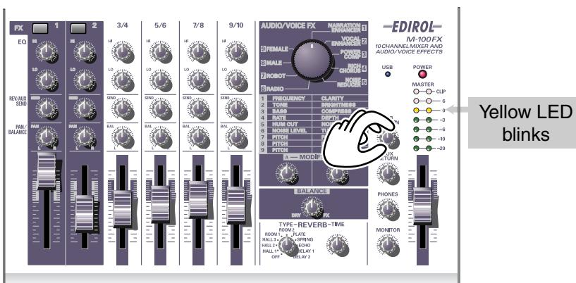
If you have connected devices to more than one line input jack (channel) and want to record them, raise the **input level faders** of all these channels to adjust their levels.
