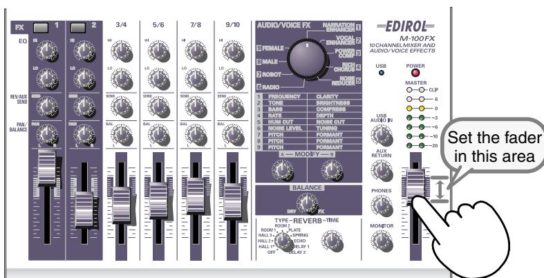
2. While playing back audio on your computer, slowly turn the **USB input level knob** toward the right to increase the level. Set the level so that the yellow LED (0 dB) of the **master volume indicator** lights occasionally.
