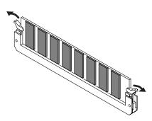
2. Remove the memory module from the socket.
