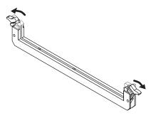
4. Paying attention to the location of the notch on the memory module and the orientation, insert it vertically within the guides at either side of the socket.
