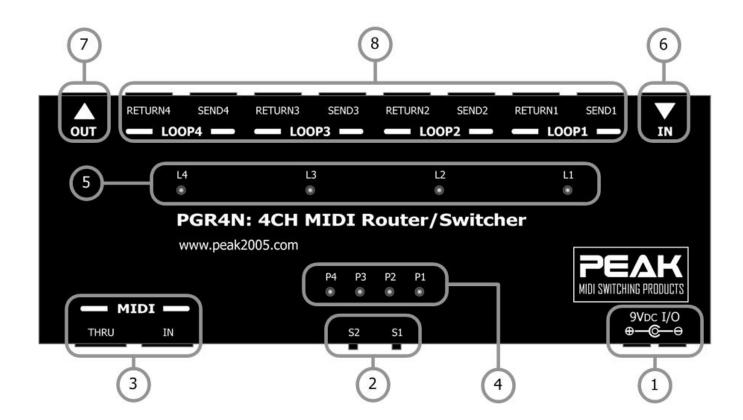
(1) **POWER In/Out:** 9V/DC, 250mA with double terminals for linking to other devices.
