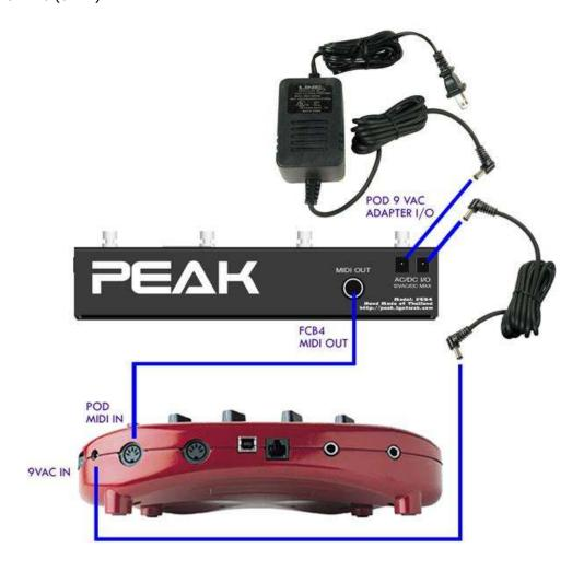
Above picture is an example that using POD 2.0 power supply with the FCB4N2 unit.
