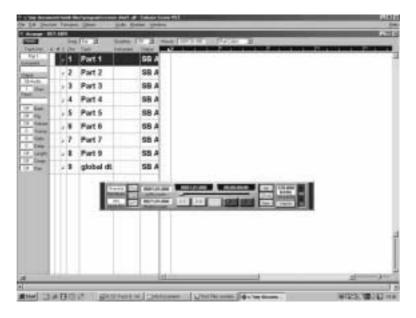
To play or edit the first Part in a multi-timbral Performance, select (highlight) the sequencer track corresponding to Part 1. Now select Part 1 on the Supernova II's front panel and change the Program assigned to Part 1 as you wish. The MIDI information transmitted by Part 1 is being re-routed back to the Supernova II Keyboard's MIDI channel for Part 1 (MIDI channel 1).
