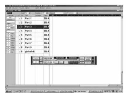
Similarly, to play or edit Part 3, first select (highlight) the sequencer track corresponding to Part 3 and then select Part 3 on the Supernova II Keyboard's front panel. Part 3 can now be edited, played or assigned its own Program using the Supernova II's front panel controls. The MIDI information transmitted by Part 3 is being re-routed back to the Supernova II Keyboard's MIDI channel for Part 3 (MIDI channel 3).
