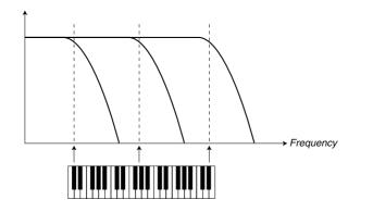
The figure shows how the Frequency1 value changes according to where on the keyboard you play when **KB TRACK** is activated.
