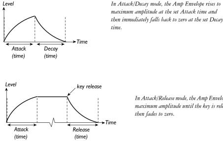
In Attack/Release mode, the Amp Envelope stays at maximum amplitude until the key is released, and then fades to zero.
