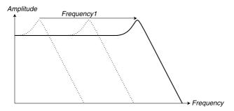
When you "open" a lowpass filter, the high-frequency content increases in the output signal.
