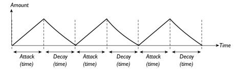
A slow looping Mod Envelope can be used for example to produce continuously sweeping pads, while shorter Attack and Decay settings can produce special effects or repetitive sounds.
