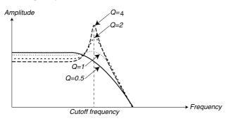
The figure shows a 24 dB lowpass filter with different resonance amounts (Q-values).
