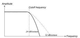
The figure shows the filter with 24 dB and 12 dB slopes.
