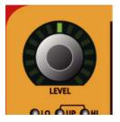
Each instrument has a **LEVEL** rotary encoder at the top. This adjusts the output level for the corresponding instrument section. The **LEVEL** encoders can be Morph controlled.
