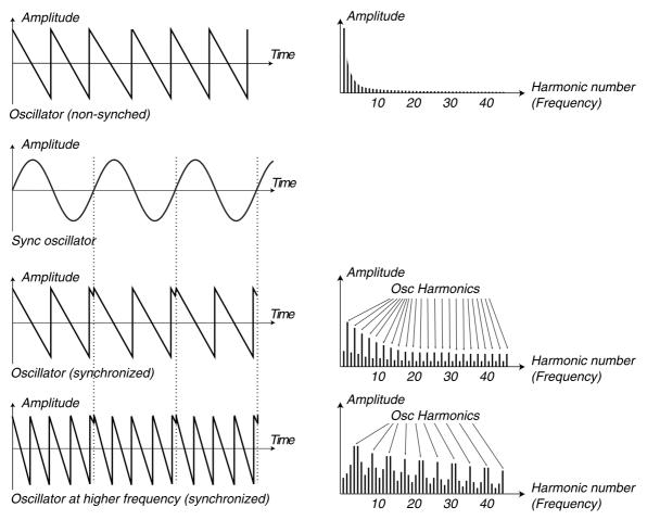
Example 1: a sawtooth wave synced by a sync oscillator. The sawtooth wave is restarted every time the sync oscillator begins a new cycle. The resulting signal gets deep resonance in its harmonics.
