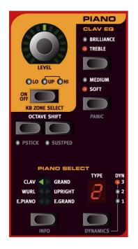
The Piano section of Nord Stage contains six Piano Categories, and each Category can contain different instrument Types. You can freely add new piano instruments via USB using the Nord Stage Manager utility (see "The Nord Stage Manager application" on page 72).
