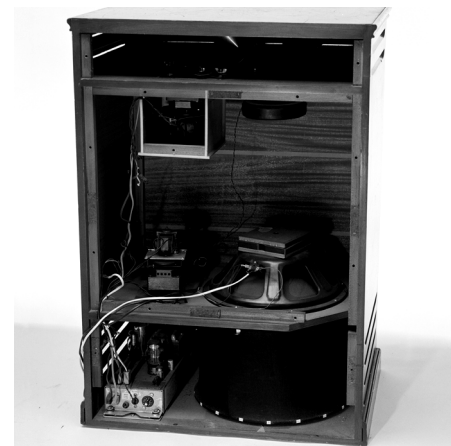
Inside a Leslie 122. Each rotor has its own motor. A 40-watt tube amplifier drives the speaker components.
