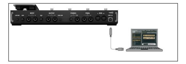
The RIG KONTROL is powered via USB. Operation is guaranteed only with a USB 2.0 controller as a single device or with self-powered USB 2.0 hubs.
