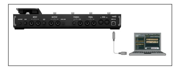
The RIG KONTROL is powered via USB. Operation is guaranteed only with a USB 2.0 controller as a single device or with self-powered USB 2.0 hubs. On Windows XP systems, Service Pack 2 or higher is required for the RIG KONTROL to work – you can find out about your Windows version in the System Properties window.
