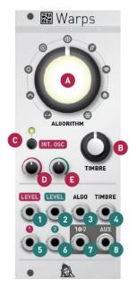
**A. Modulation algorithm.** This knob selects which signal processing operation is performed on the carrier and modulator. The algorithms are described in further details in the next section.
