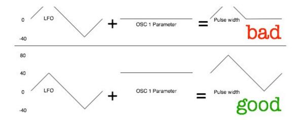
Quirk ahoy! The modulation amount of the last patch cord is adjusted by the modwheel. Huh? Let's say you set patch cord 12 to go from LFO 1 to the oscillators fine pitch with an amount of 16:
