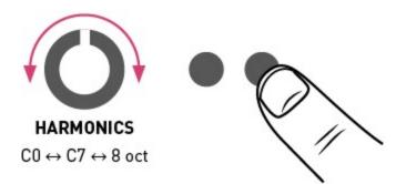
After having turned the **HARMONICS**, **TIMBRE** or **MORPH** knob to adjust a setting, the position of the knob might no longer match the original value of the corresponding parameter. When this happens, the response curve of the knob is modified to account for this discrepancy, until the position of the knob and the parameter perfectly line up again!
