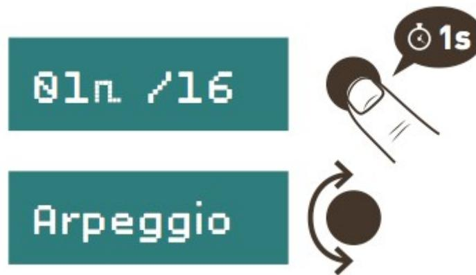
Each “feature” of the MIDIpal can be seen as an independent “app”. Only one app can be running at a time - that is to say, you cannot run an arpeggiator, a drum sequencer and a MIDI monitor on the same unit! To select the app to use, keep the encoder pressed. The name of the current app is shown on the screen.
