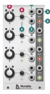
**A. Channel polarity and gain.** At 12 o'clock, the channel is muted. Turn clockwise to amplify, turn counter-clock- wise to amplify and invert.
