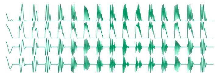
This waveform family simulates the sound of a trapezoidal pulse wave processed by a low-pass, peaking, band-pass, or high-pass resonant filter. The parameter controls the cutoff frequency of the filter. **pkzpulse** is particularly good at recreating the dirty, saturated sound, of a sawtooth filtered by the least academic of the 2-pole analog filters.
