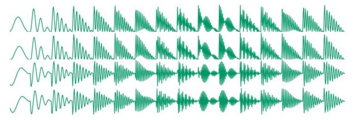
This waveform family directly simulates the sound of a sawtooth wave processed by a low-pass, peaking, band-pass, or high-pass resonant filter. The parameter controls the cutoff frequency of the filter.
