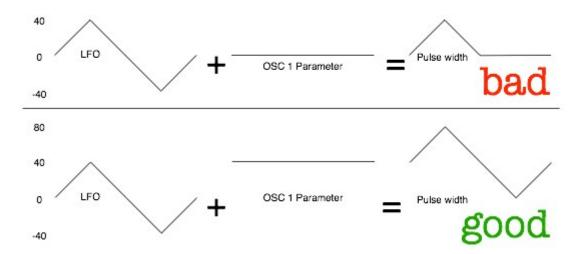
LFOs, pitch-bend and MIDI note number modulations are bipolar. If you are used to electronics/Modular speak, it is equivalent to say that the LFOs are always "AC-coupled" instead of "DC-coupled".
