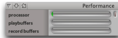
Figure 10-6: When adjusting the buffer size to reduce monitoring latency, watch the 'processor' meter in Digital Performer or AudioDesk's Performance Monitor. If you hear distortion, or if the Performance meter is peaking, try raising the buffer size.
