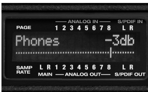
Figure 6-3: For many settings, the LCD “zooms in” on the setting as you adjust it.
