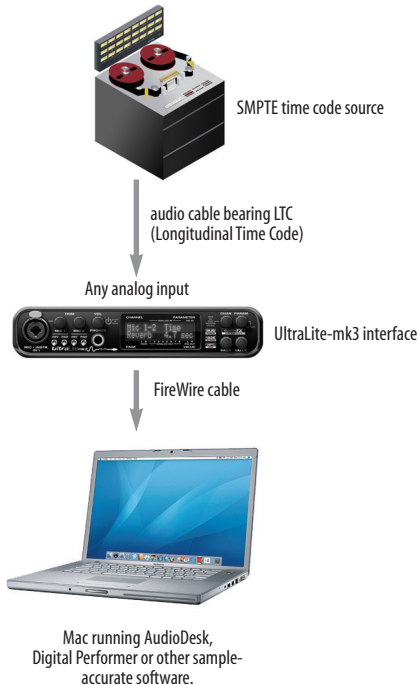
Figure 12-3: Connections for synchronizing the UltraLite-mk3 directly to SMPTE time code.
