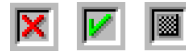
Figure 10-13: A red “X” means data will be filtered. A green check mark means the data will not be filtered. A “hatched out” box indicates that data is both filtered on one or more channels and not filtered on one or more channels. The non-channelized filters will never show the hatched-out box, since they apply to all channels.
