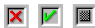
Figure 7-13: A red “X” means data will be filtered. A green check mark means the data will not be filtered. A “hatched out” box indicates that data is both filtered on one or more channels and not filtered on one or more channels. The non-channelized filters will never show the hatched-out box, since they apply to all channels.
