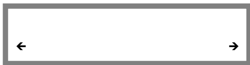
Figure 11-1: The left and right arrows indicate other windows to the left or right, which you can scroll to with the CURSOR knob.
