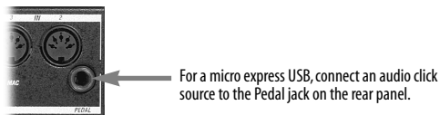
Figure 2-8: Connecting an audio click input. Only the Pedal A input on the rear panel of the MIDI Timepiece AV can be used as a click input.
