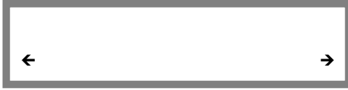
Figure 17-1: The left and right arrows indicate other windows to the left or right, which you can scroll to with the CURSOR knob.
