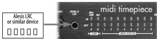
Figure 2-15: Connecting an Alesis LRC remote controller (or any LRC-compatible MMC controller) to a MIDI Timepiece AV.
