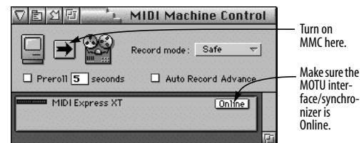
Figure 5-4: Performer 6.0 and Digital Performer 2.0 (or later) automatically configure their MIDI Machine Control window when a MOTU MIDI interface/synchronizer is present in the current FreeMIDI configuration. They automatically detect the interface/synchronizer's MMC device ID.
