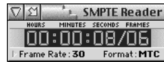
Figure 11-1: The SMPTE Reader provides a running update of your MOTU interface while it is generating or converting time code.
