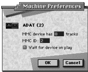
Figure 10-18: To set machine preferences, click the panel of the ADAT you want to set preferences for and choose the Set Machine Preferences command from the mini-menu in the title bar of the window.
