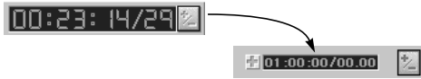
Figure 10-3: Click the button as shown to type in a global SMPTE offset for your MOTU interface.
