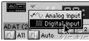
Figure 10-15: To choose the record source (either the analog or digital inputs on the ADAT), choose the desired source from the pop-up menu as shown.
