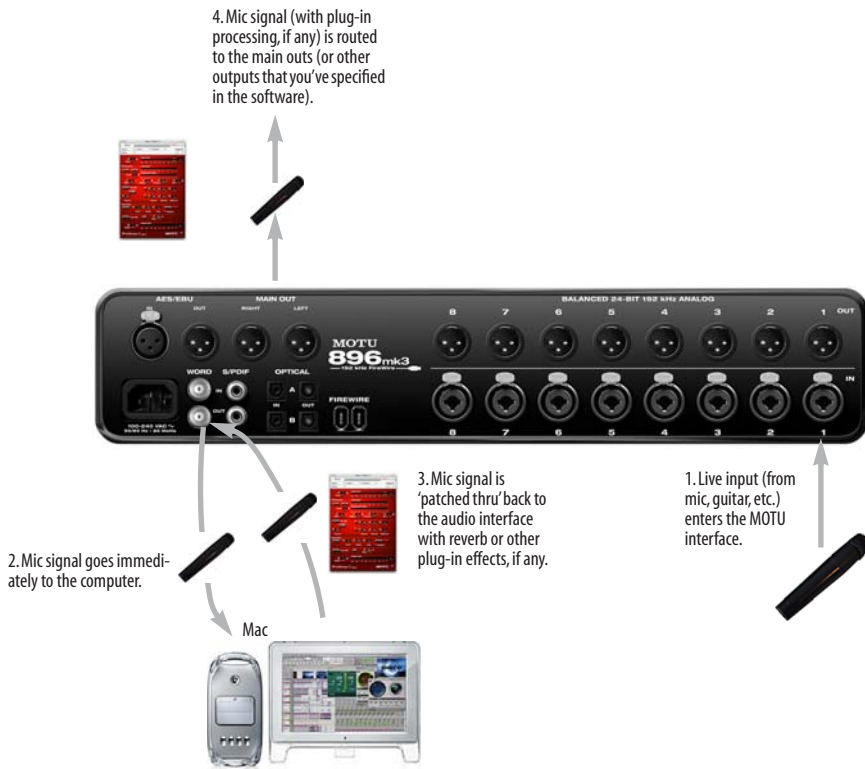
Figure 10-1: There are two ways to monitor live audio inputs with an 896mk3: 1) through the computer or 2) via CueMix FX hardware monitoring. This diagram shows method 1 (through the computer). When using this method, use your host software's buffer setting to reduce the slight delay you hear when monitoring the live input, but don't lower it too much, or your computer might get sluggish.
