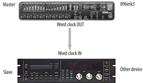
Figure 3-17: Slaving another digital audio device to the 896mk3 via word clock. For the 896mk3 clock source, choose any source besides word clock, as it is not advisable to chain word clock.
