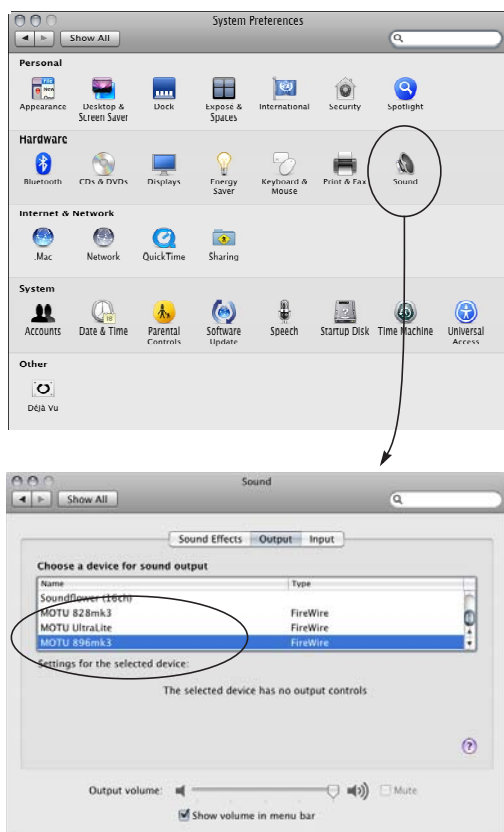
Figure 5-2: The Mac OS X sound preferences let you use the 896mk3 for general stereo audio input and output for your Mac.
