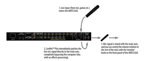
Figure 5-3: This diagram shows the signal flow when using CueMix<sup>TM</sup> Plus no-latency monitoring. Notice that this method does not allow you to process the live input with plug-ins in your audio software while it is being monitored. You can, however, add effects later — after recording the live input as a disk track. CueMix<sup>TM</sup> Plus lets you hear what you are recording with no delay and no computer-based effects.
