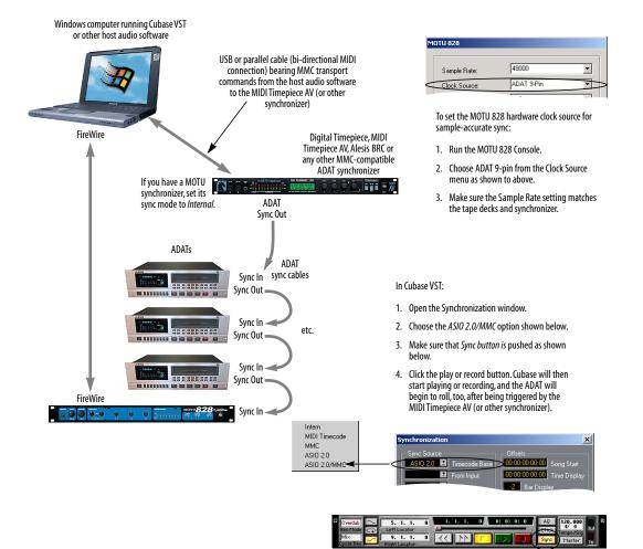
Figure 4-10: Connections for sample-accurate sync between one or more ADATs and the MOTU 828.
