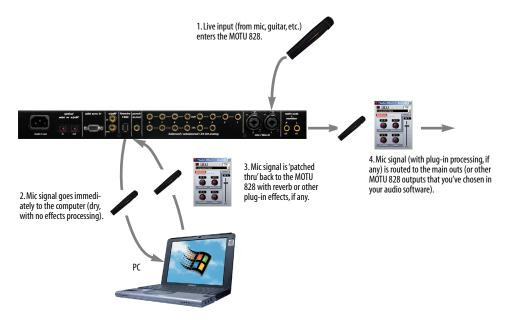
Figure 5-2: There are two ways to monitor live audio inputs with the MOTU 828: 1) through the computer or 2) via CueMix<sup>TM</sup> Plus hardware monitoring. This diagram shows method 1 (through the computer). When using this method, use the MOTU 828's 'Samples Per Buffer' setting to reduce the slight delay you hear when monitoring the live input, but don't lower it too much, or your computer will act sluggish.
