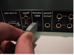
Figure 4-1: Connecting the MOTU 828 to the computer.
