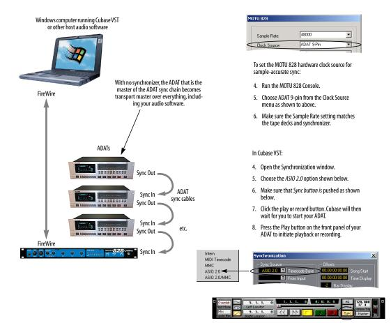
Figure 4-10: Sample-accurate sync without an ADAT synchronizer.
