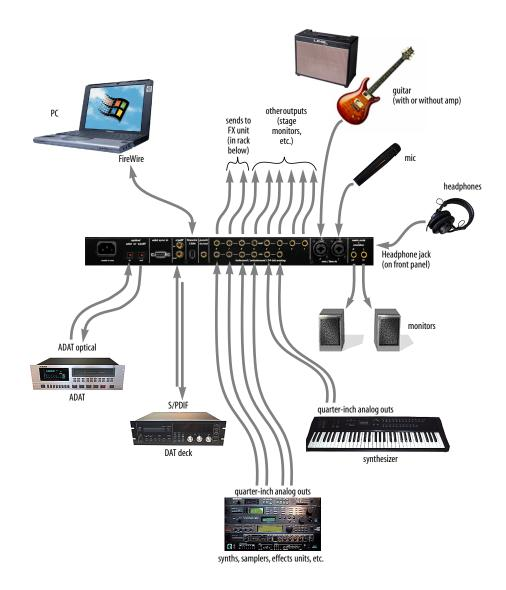
Figure 4-3: A typical MOTU 828 studio setup.
