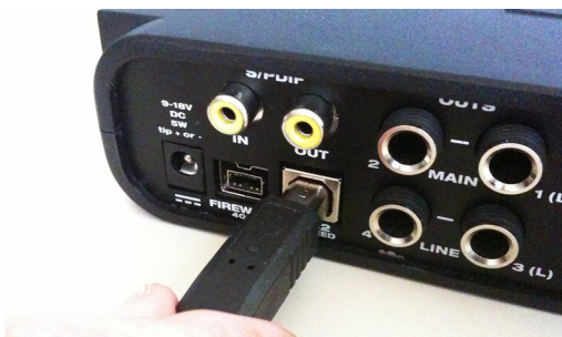
Figure 4-1: Connecting the 4pre to the computer via USB.
