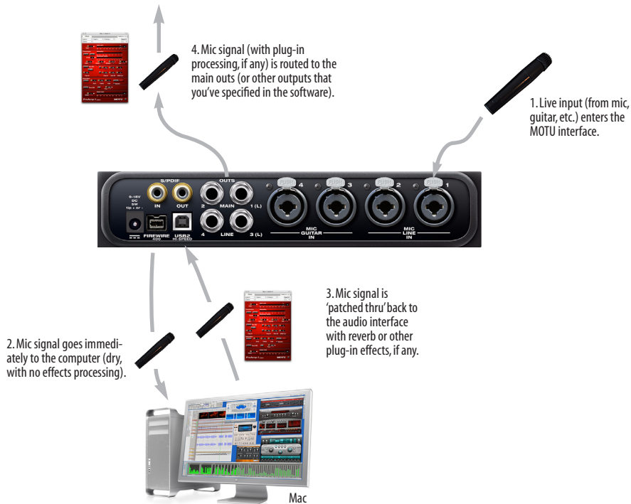
Figure 8-1: There are two ways to monitor live audio inputs with an 4pre: 1) through the computer or 2) via CueMix hardware monitoring. This diagram shows method 1 (through the computer). When using this method, use your host software's buffer setting to reduce the slight delay you hear when monitoring the live input, but don't lower it too much, or your computer might get sluggish.
