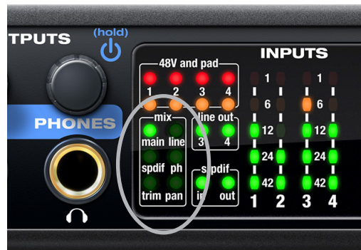
Figure 6-3: The Mix LEDs indicate which mix you are controlling with the front panel.
