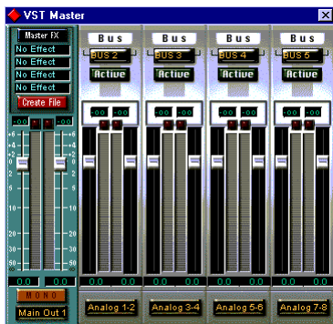
Figure 8-5: Use the output buttons at the bottom of each channel strip, including the master fader, to assign 24i outputs to buses. You can then assign channels in the Monitor window to each bus as desired.
