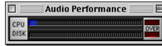
Figure 8-6: Keep the Audio Performance window open to keep tabs on your computer's processing power and hard disk performance.
