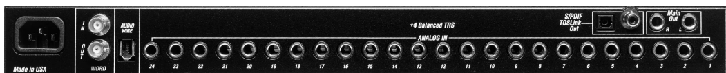
Figure 6-3: The 24i gives you 24 inputs and stereo main outputs in three formats: 24-bit analog, optical S/PDIF and RCA S/PDIF.
