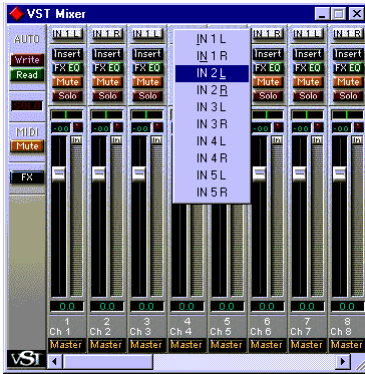
Figure 8-4: Assigning a 24i input to a VST audio channel: control-click the input button at the top of the channel strip.
