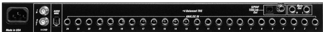
Figure 5-3: The 24i gives you 24 inputs and stereo main outputs in three formats: 24-bit analog, optical S/PDIF and RCA S/PDIF.
