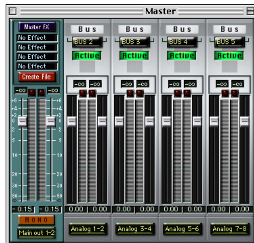
Figure 10-5: Use the output buttons at the bottom of each channel strip, including the master fader, to assign 24i outputs to buses. You can then assign channels in the Monitor window to each bus as desired.
