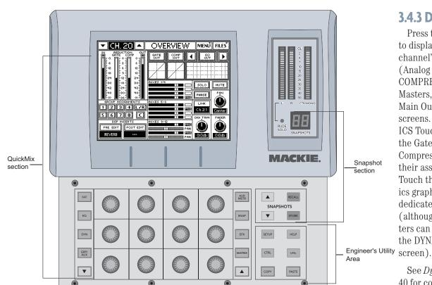
Figure 3-5 QuickMix Section
