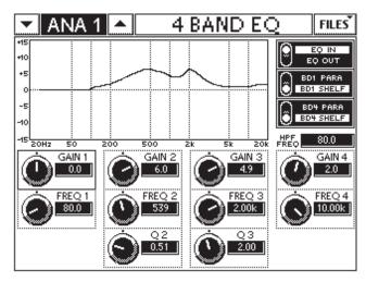
Figure 6-12 Analog Channel 4-BAND EQ
