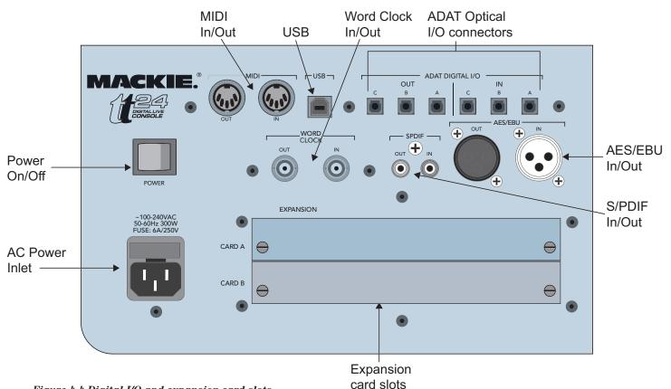
Figure 4-4 Digital I/O and expansion card slots
