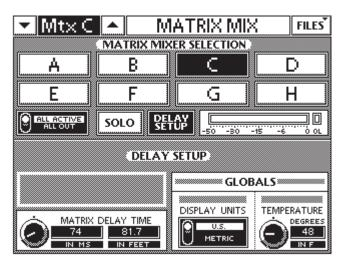
Figure 6-24 MATRIX MIX DELAY SETUP Touchscreens
