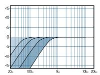
The HPF (high pass filter) switch, often referred to as a low cut filter, cuts bass frequencies at a rate of 12dB per octave below a swept-select point, ranging from 30Hz–800Hz. Using HPF will clean out the "mud" in your mix, can help reduce the possibility of feedback in live situations, and help to conserve amplifier power.
