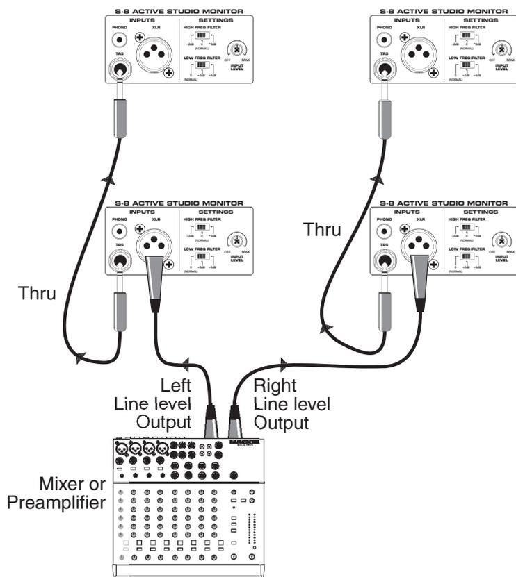
Note: Use stereo 1/4" TRS plugs for the "Thru" connections. If you use mono 1/4" TS plugs, you will unbalance the XLR connections and suffer a drop in signal level of 6 dB.
