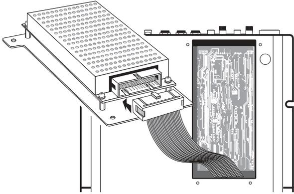
5. Fit the card in place, with its large plate flush with the bottom panel, and its FireWire connectors lined up in the holes of the d.2 rear panel. Secure the bottom plate in place using the four screws you took out in step 2. Fit one other screw in the hole between the two FireWire connectors. There will be one screw left over to put under your bed.
