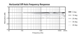
Frequency response is measured on-axis at a distance referenced back to 1m at 1-watt drive. Shown as a half space  $(2\pi)$  environment.
