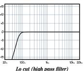
Lo cut (high pass filter) 18dB/oct. at 75hz
