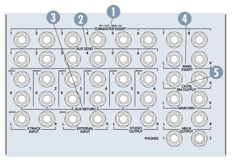
right return inputs and end up centered in your stereo image. When a jack is plugged into the Right input of the return, this mono feature is disabled: the left input is fed to the left return, and the right input is fed to the right return.
