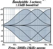
Bandwidth: 3-octave; ±15dB boost/cut When you put these consoles on the test bench, you see that the bandwidth of their EQ is simply too narrow — often around one octave. This is OK for extreme adjustments in live situations, but that's about it. It's just not wide enough to gently alter the multiple octaves that voices and instruments span.
