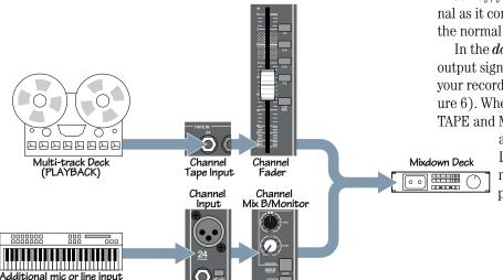
Figure 6: FLIP/MIX-B signal path during mixdown showing additional input ("flip" switch down)
