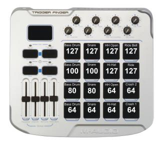
Here, each pad has individual note and Velocity Lock assignments. This allows you to play with the precision of the spread mode while having access to more than one sound. You can, of course, assign any sound to a pad—this is merely an example.
