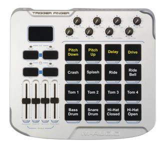
The yellow labels indicate pads that are not transmitting MIDI note data—they're only sending MIDI controller messages. These messages are being use to control the pitch of the kit, the reverb send, and the drive of a distortion plug-in.
