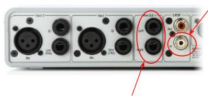
From the Mbox Mon Out jacks, connect to the Left and Right inputs for your powered speakers or monitoring system
