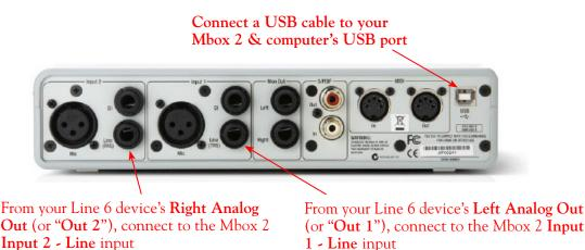
You will still use the Mbox 2 **Mon Outputs** (or Headphone Output) to hear playback of all Pro Tools LE audio. The Line 6 Hardware/GearBox audio will be mixed with the Pro Tools LE audio as well. Therefore, if you are using headphones, you'll want to plug them into the Mbox 2 headphone jack to hear everything:
