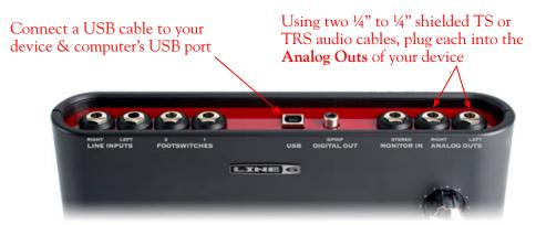
\*Note - If you are using a GuitarPort device, the Analog Outs are the RCA style jacks labelled "L" and "R". If using a TonePort UX8, you should connect to the "Out 1" and "Out 2" jacks on the back.
