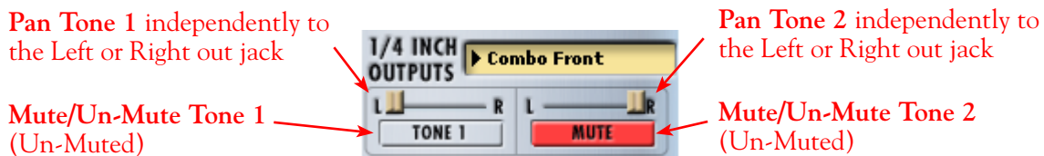
1/4 Inch Out controls are displayed when one of the Live modes is selected
