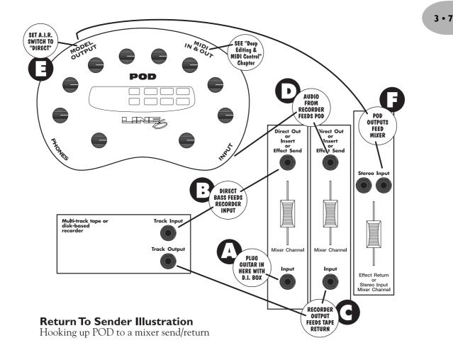
Plug the bass into your DI. Plug the DI into a mixer channel with a direct out. Set the trim on your channel so your input levels look good. Plug the direct output
