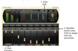
In the modifier button area, just above the fader, you will see the name of the parameter that is assigned to that position in the soft row. Clicking on any of these parameter buttons reveals a list of all the algorithm's parameters. Select a parameter (or "no selection") from the list, and that parameter is then assigned to the soft row. The assigned parameter is still available on its original edit page, but now it appears in the soft row as well.
