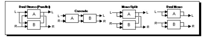
Generally, the **Effects LvI/Bal** parameter (Page 1, Edit knob 3) controls the balance of the two effects in each dual program. In the cascade variations, rather than simply controlling balance, the knob varies the amount of the first effect or dry signal which is fed into the second effect.
