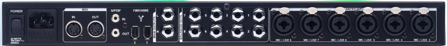
MIDI In/Out S/PDIF In/Out FireWire® 400 Ports Stereo Main (Control Room) Outs 8 Analog TRS Outputs Combi XLR/TRS Balanced Mic/Line Inputs
