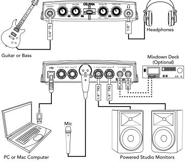
**NOTE:** When connecting to the **Instrument** input, the **LINE 1** input will be deactivated. When connecting to the **LINE 2** input, the **Mic** input will be deactivated.
