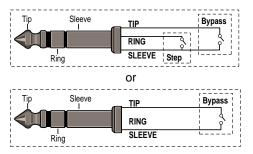
When shipped, Alex is configured to use push on/push off type switches. You can change this configuration to allow the use of momentary contact switches by performing the following procedure:
